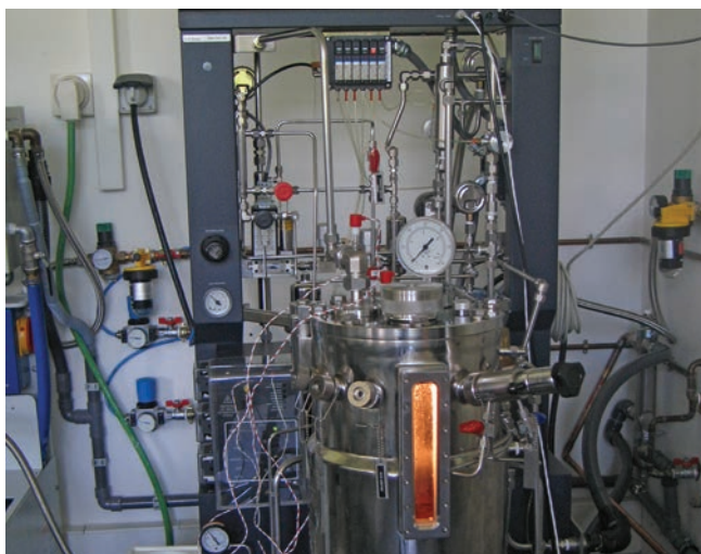
Fig. 2 Pilot plant fermenter to obtain bioethanol
