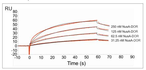
**Figure 5**- Interaction between LC3 (Ligand) and different concentrations of NusA-DOR (analyte). Representation of the interaction with LC3 on Channel 1 (300 RUs). Red lines represent the experimental interactions measured in a Biacore T100. Dotted lines correspond to the curves used for fitting the data.
