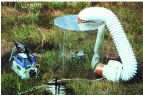
Soil respiration measurements in a Hungarian grassland (part of the “CarboEurope” European project).
