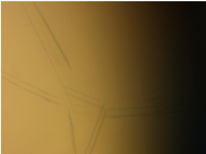
Figure 9- Needle-like crystals from the LC3-DOR peptide complex (1:1).
